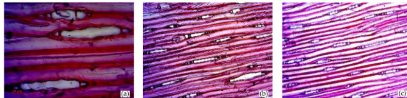
Figure 2. The damage of the ray cells on the tangential surface of the radial and tangential boards (a) under high magnification ( \times 40 ), and (b,c) under low magnification ( \times 10 ).
